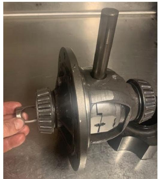
5. Reach in through the recess in the cam gears and rotate the thrust block so that the hole in the middle lines up with the cam gear recesses.
