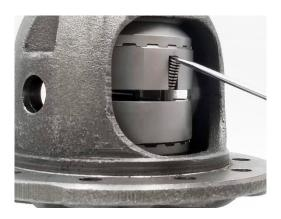
8.) <u>Install the Pins and Springs:</u> Pins go in the hole, springs go in the slot. The nub on pin retains bottom loop of spring. It's helpful if you use the nub on the pin to hold the spring in place, then use a small screw driver to compress the spring and pop it into the slot. It's critical to install the pins and springs in the correct orientation. Failure to install in the correct orientation could lead to severe damage in the differential.
