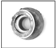
4.) <u>Thrust Washers:</u> Install new or existing thrust washers onto the backs of the axle gears and press them into the grease to help hold them in place.
